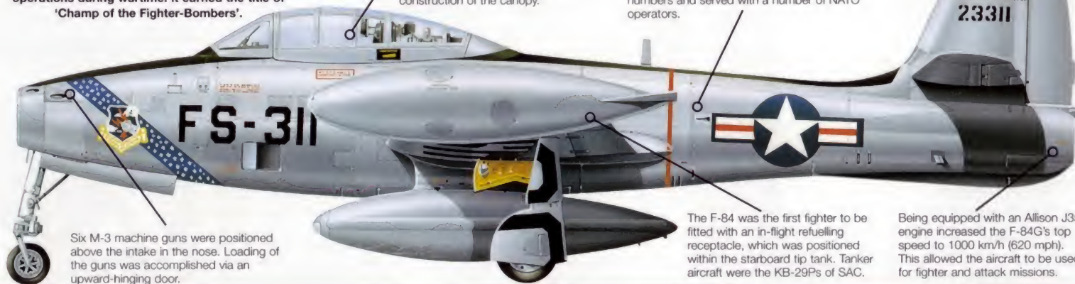
The cockpit was enclosed under a sliding canopy. Later models were fitted with bracing struts to increase the strength of the hood against bird strikes. This also considerably eased construction of the canopy.
